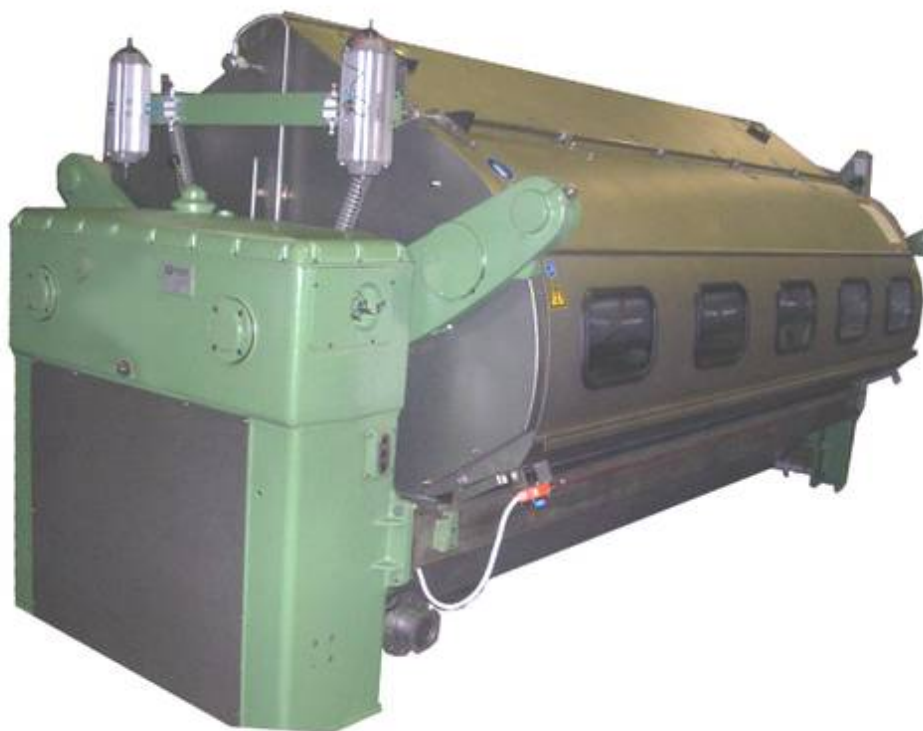
Jigger with roller width 3600mm
